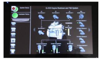
Ex SCS features a touchscreen Human Machine Interface (HMI) that displays the current status of the safety shutdown system.
