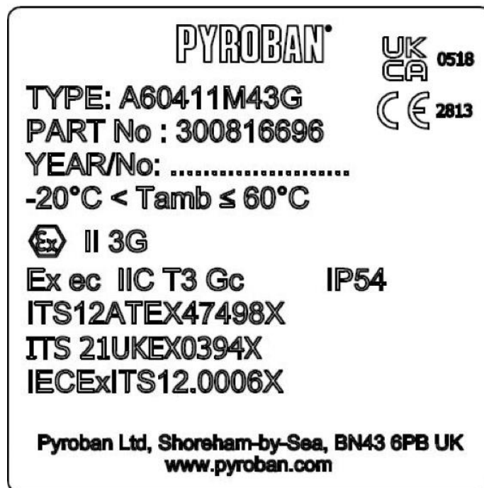
Figure 5 – 60 kVA Alternator Hazardous Area Rating Label
