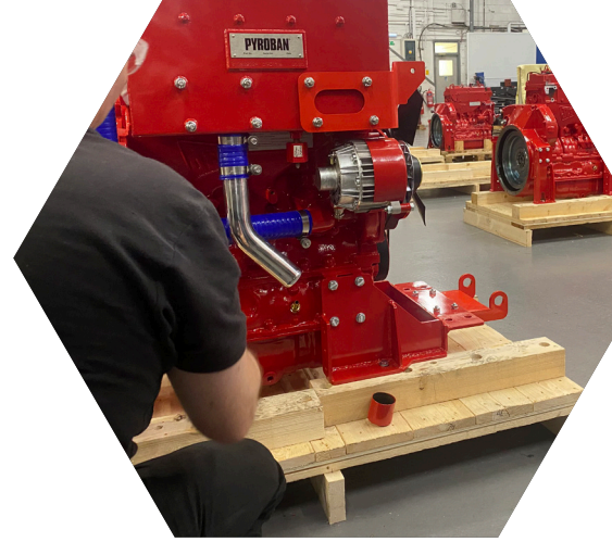
Explosion proof kits being fitted at the UK Pyroban factory for operations in the Middle East
